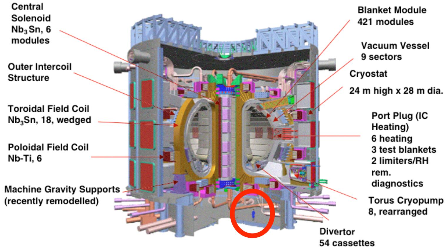
Figure 1. ITER tokamak and major components.
