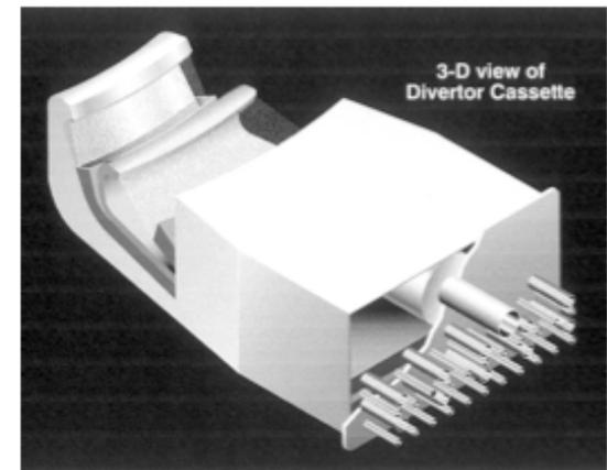
Fig. 1. Example of an advanced liquid surface divertor module.
