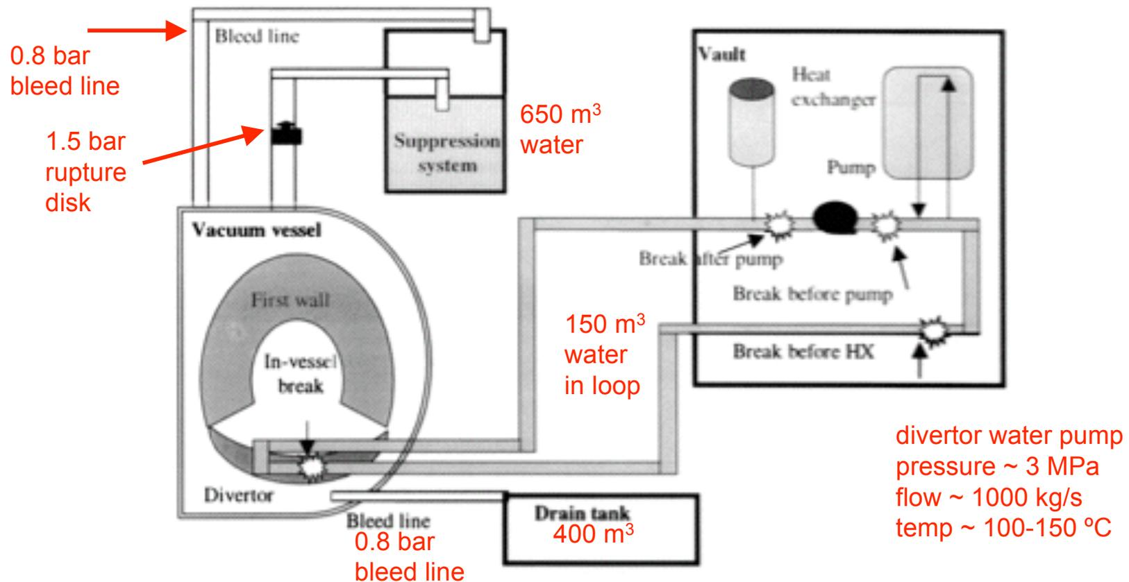
Fig. 1. Plant scheme and breaks' locations.
