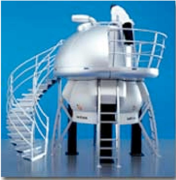
**A 900-MHz nuclear magnetic resonance device.**
