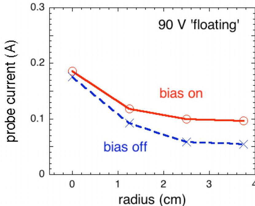
current drawn by floating electrodes ~ 1 Amp, compared with ~8 Amp for + bias with respect to vessel => uses less power
