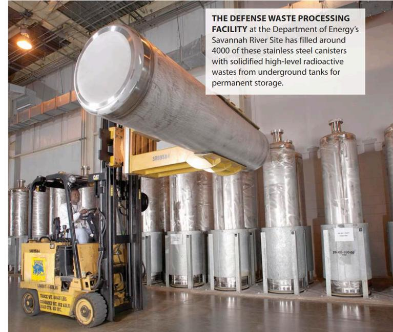
**THE DEFENSE WASTE PROCESSING FACILITY** at the Department of Energy's Savannah River Site has filled around 4000 of these stainless steel canisters with solidified high-level radioactive wastes from underground tanks for permanent storage.
